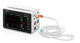
With the portable module rack, N1 can also support extended modules, including sidestream/microstream/mainstream CO<sub>2</sub> and PiCCO modules, thus meeting the requirements of different transport scenarios.
